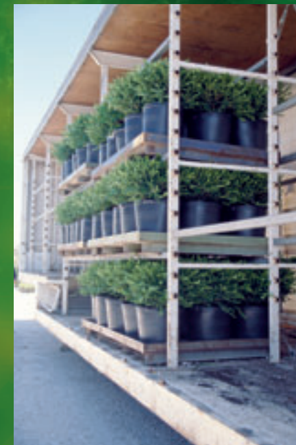
Curtain sidewalls on trailers can reduce loading and unloading time.
